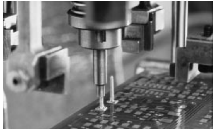
Continuous Surf-Shooter SMT™ Connector Separated and Presented to Vacuum Pick-up
