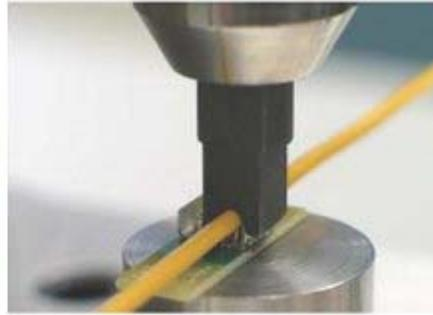
The new Zierick process begins with the terminal being placed on, and soldered to, the SMT board together with the other required components. After the assembly goes through reflow, it is moved to the terminating machine which feeds the wire into the terminal and crimps the terminal walls over the wire. In the process, the insulation piercing spikes penetrate into the wire without the necessity of
