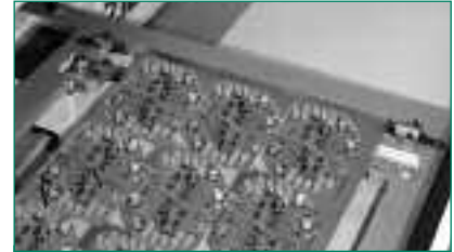
Zierick's Model 9700 X,Y Terminal Insertion System is fully automatic, with a machine cycle rate of over 5,000 pph.
